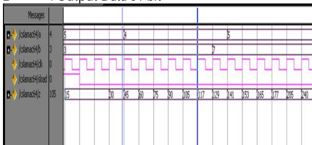
Fig 9: Simulated Waveform of Pipelined Booth Wallace MAC Unit
